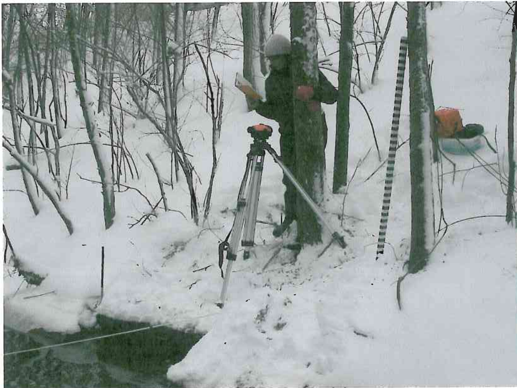
Figure 2. Measuring the river cross-section at transect-1 using a transect and stadia rod.
