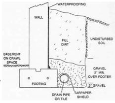
cases, the exterior wall will require excavation down to the footer and a functioning drain installed.
