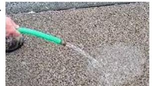
Pervious concrete allows water to percolate into the ground, whereas conventional concrete and asphalt do not absorb water
